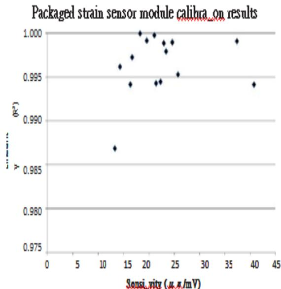
Fig. 11. Calibration results on strain sensor front-end modules.
