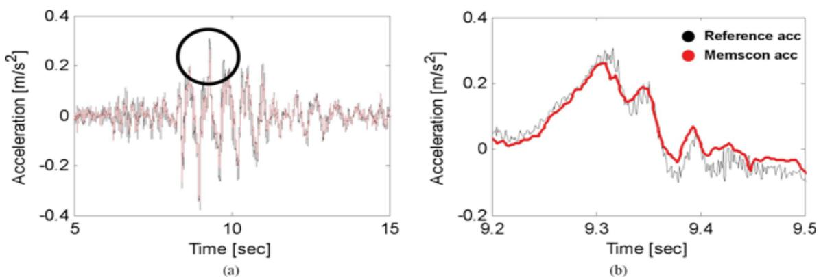
Fig. 9 (a) Wireless sensor module acceleration signal output (lowpass-filtered for noise reduction) on full-scale model with simulated earthquake and comparison to reference accelerometer (traditional piezoelectric uniaxial-wired accelerometer). (b) Enlargement of the peak of the signal.
