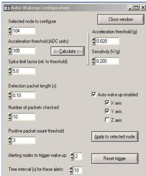
Fig. 7. User interface showing per-node tunable parameters of the earthquake wake-up procedure
