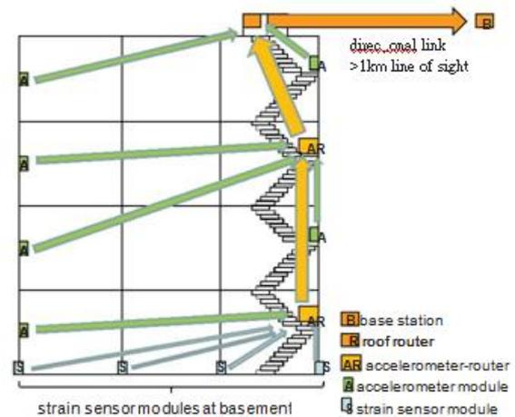
Fig. 1. Network architecture of the monitoring system in a building.
