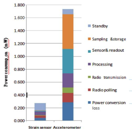
Fig. 8. Sensor module power consumption results.
