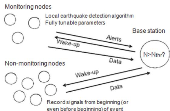
Fig. 6. Diagram of distributed earthquake wake-up procedure.
